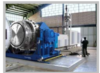
KraussMaffei Berstorff extrusion line for extra-large pipe with a 36D single-screw extruder and a spiral distributor pipehead
